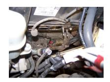
**3.** Now install driver side GIBSON header and gasket using stock hardware to the head and torque the header to 30-35 ft/lb. Now re-install dipstick and EGR tube back to there original locations on the vehicle.
