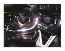
**7.** Re-install Y-pipe assembly to the GIBSON headers and torque to 30-35 ft/lb.
