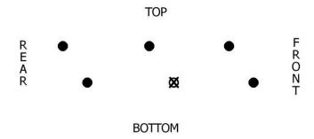
$\pmb{6}$ . Now install passenger side GIBSON header, gasket, stock hardware, the supplied 8mm bolt and washer to the head and torque the header to 30-35 ft/lb.
