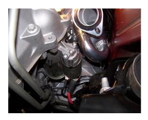
17. RE-CONNECT THE EXHAUST SYSTEM TO THE NEW HEADERS USING THE HARDWARE PROVIDED.
