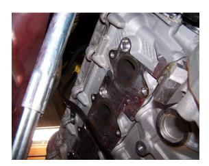
9. ON THE PASSENGER SIDE, AGAIN WORKING UNDERNEATH AND FROM THE TOP, REMOVE THE NUTS ATTACHING THE MANIFOLD TO THE HEAD. REMOVE THE MANIFOLDS ATTACHING STUDS. (NOTE: MUST REMOVE ALL UPPER AND LOWER STUD BEFORE MANIFOLD WILL COME OUT.)
