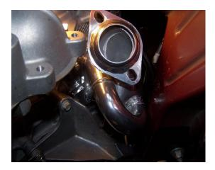
16. ONCE ALL BOLTS ARE SNUG. LOWER MOTOR BACK DOWN AND RE-TORQUE ENGINE MOUNT. TORQUE DOWN BOLTS STARTING WITH THE CENTER BOLTS FIRST. RECOMMENDED TORQUE SPECS. ARE 25-30 FOOT POUNDS OF TORQUE.
