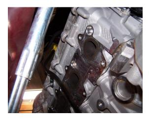
9. ON THE PASSENGER SIDE, AGAIN WORKING UNDERNEATH AND FROM THE TOP, REMOVE THE NUTS ATTACHING THE MANIFOLD TO THE HEAD. REMOVE THE MANIFOLDS ATTACHING STUDS. (NOTE: MUST REMOVE ALL UPPER AND LOWER STUD BEFORE MANIFOLD WILL COME OUT.)
