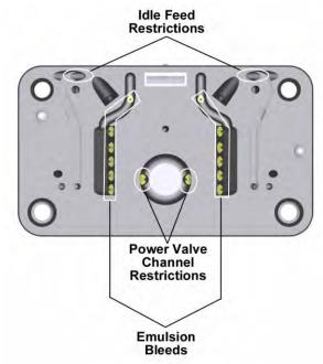
3 Circuit Billet Metering Block (Front) Model 4500 Ultra HP DOMINATOR Figure 9
