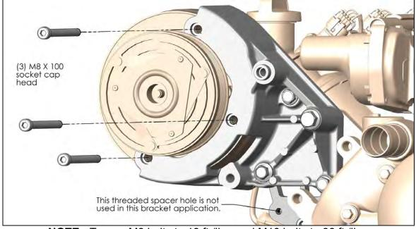
NOTE: Torque M8 bolts to 18 ft./lbs. and M10 bolts to 36 ft./lbs.
