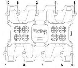
**Manifold Tightening Sequence**
