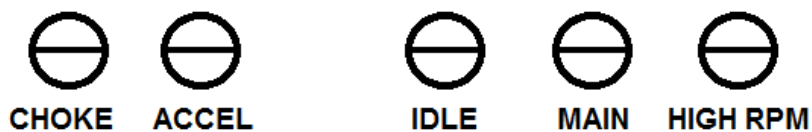
Figure 19: Adjustment Potentiometer Settings for Initial Startup
