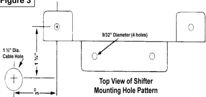
5. Install the rubber grommet in the 1 1/2" cable hole located in the floor.
