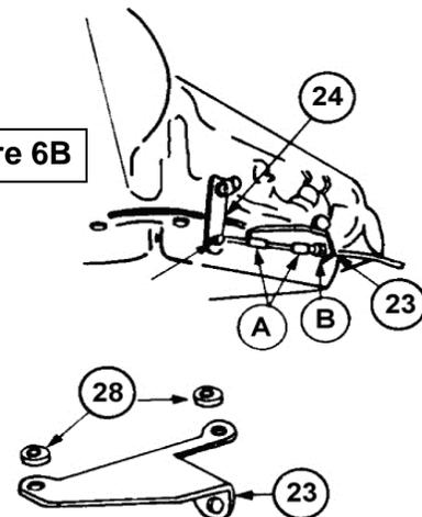
10. Remove the tape from the cable and reinstall one nut and flat washer **B** on the shifter cable. Route the shifter cable through the bracket and reinstall the other flat washer, nut **B**, and two rubber boots **A** (See Figure 2, 6A or 6B).
