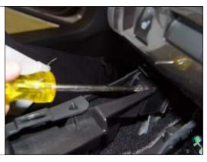
**STEP 7.** Remove the rubber tray in the center console storage box.
