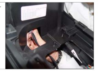
**STEP 29.** Re-install the screws in the bottom of the center console storage box.
