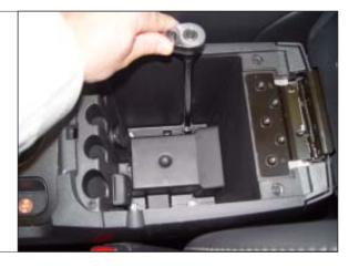
**STEP 9.** Raise the center console to access and disconnect the center console storage box lighting connection and any additional wiring connection clips.
