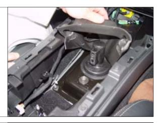
**STEP 13.** Unscrew rear mounting nut. TOOLS: ratchet, long extension and 13mm socket
