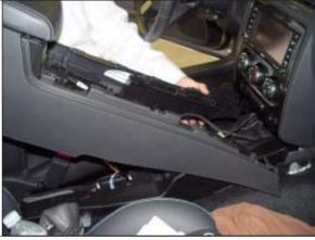
**STEP 28.** Raise the center console to access and reconnect the center console storage box lighting connection and any additional wiring connection clips.
