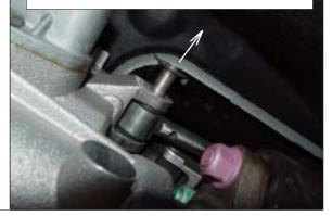
**STEP 17.** From inside the vehicle, lift up on the shifter assembly to access the lower change rod connection bolt and remove both bolt and then shifter from vehicle.
