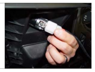
**STEP 5.** Disconnect the cupholder lighting connection and remove the center console trim/cupholder plate.
