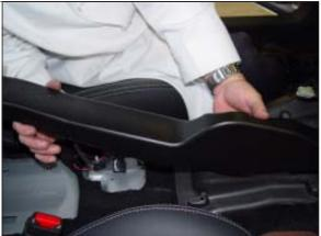
**STEP 12.** Remove the wiring routing ties from the rubber shift boot cover and remove cover.
