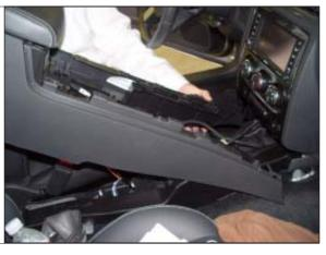
**STEP 11.** Remove rear A/C duct by pulling rear ward.
