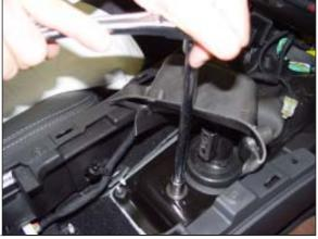
**STEP 14.** Unscrew six tunnel cover mounting nuts. TOOLS: ratchet, long extension and 10mm socket
