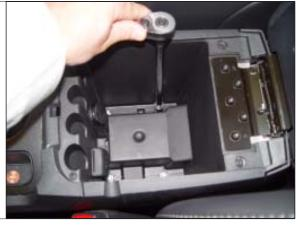
**STEP 30.** Replace the rubber tray in the center console storage box.
