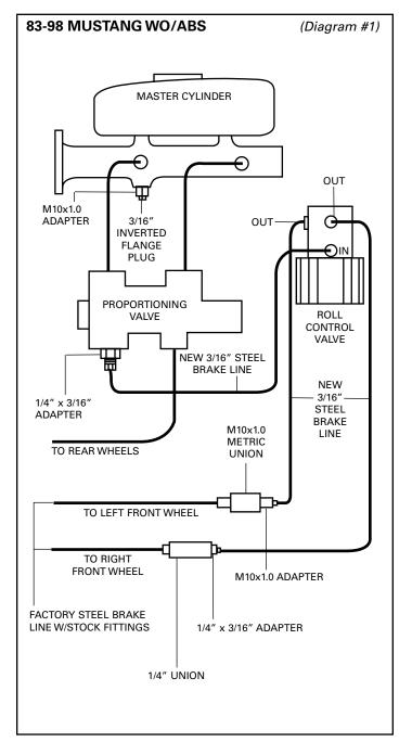
adapter. Plumb the other end of this line to the remaining "outlet" port on the Roll/Control unit.
