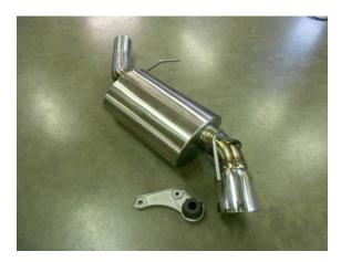
1) Place the new Hurst muffler units next to the factory unit and swap the rear hanger mounts from the stock muffler to the Hurst assemblies.
