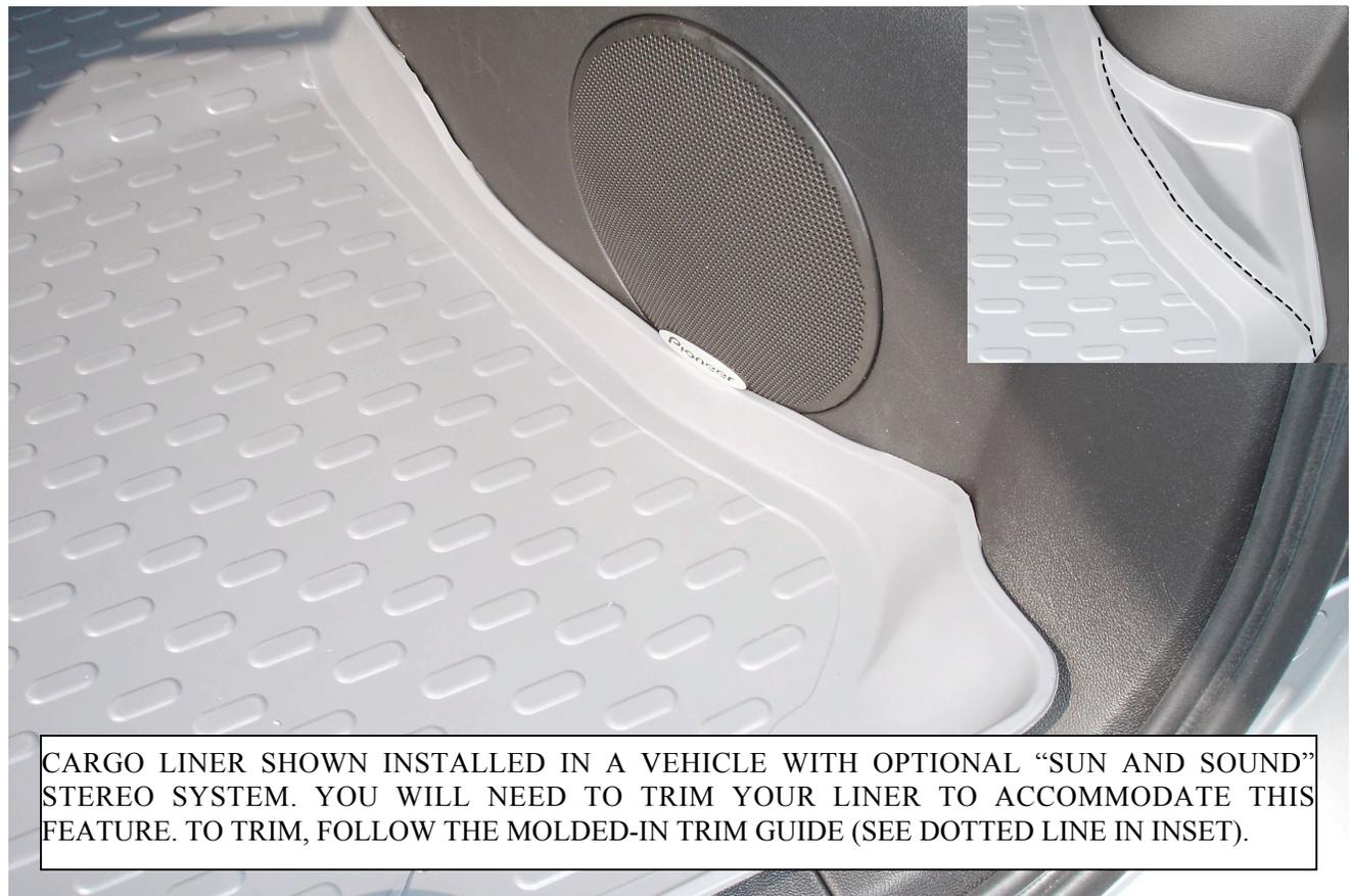
CARGO LINER SHOWN INSTALLED IN A VEHICLE WITH OPTIONAL “SUN AND SOUND”
