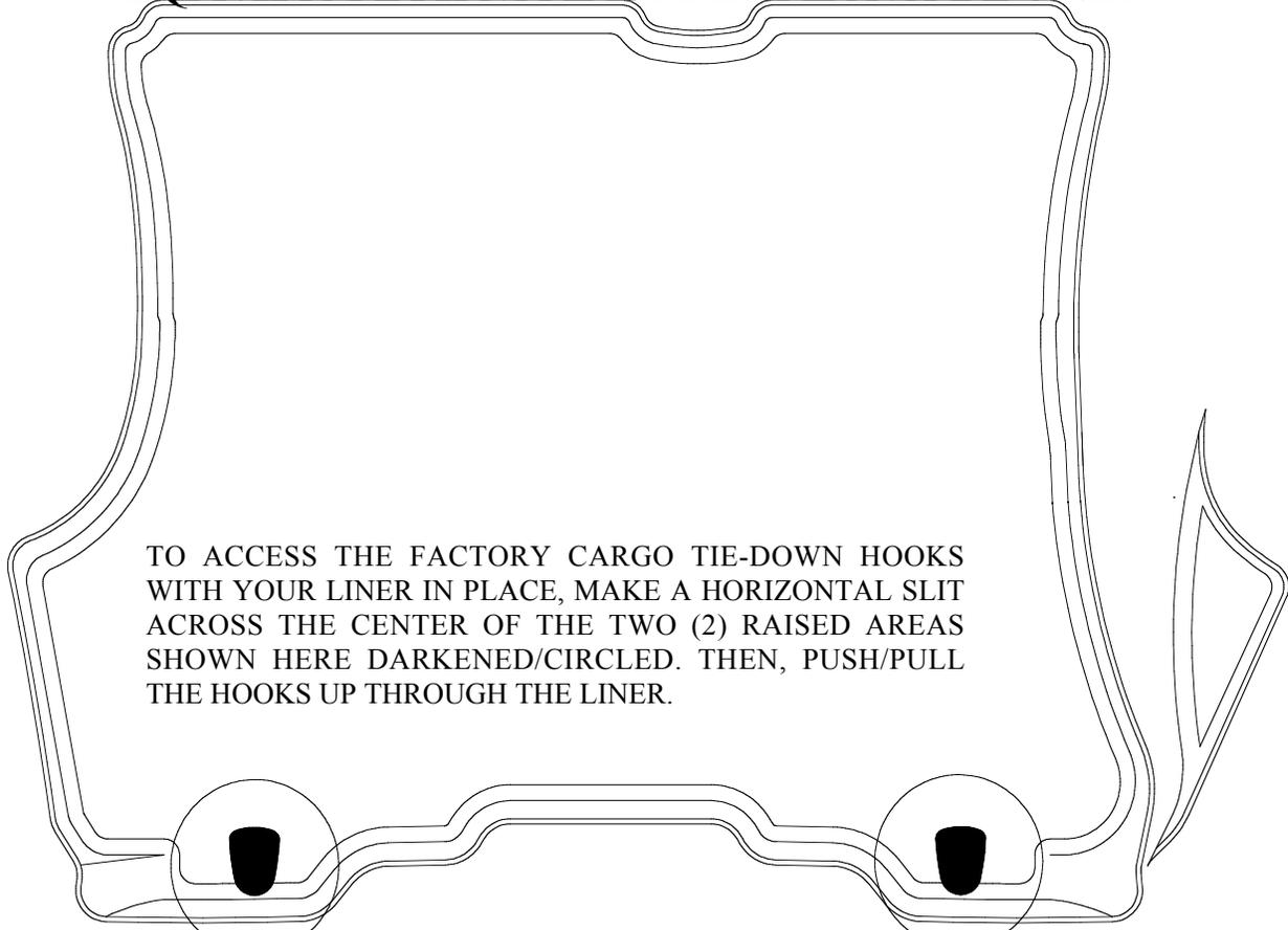
TO ACCESS THE FACTORY CARGO TIE-DOWN HOOKS WITH YOUR LINER IN PLACE, MAKE A HORIZONTAL SLIT ACROSS THE CENTER OF THE TWO (2) RAISED AREAS SHOWN HERE DARKENED/CIRCLED. THEN, PUSH/PULL THE HOOKS UP THROUGH THE LINER.
