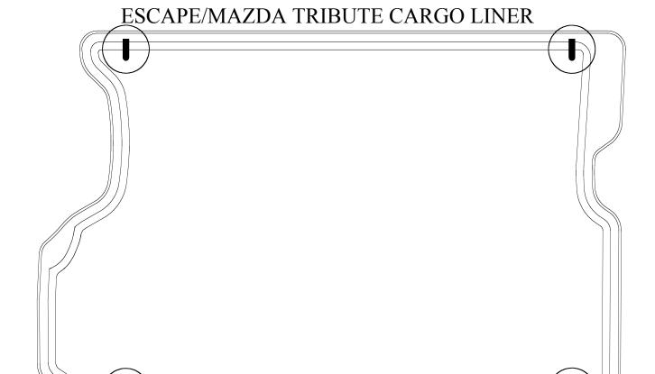
TO ACCESS THE FACTORY CARGO TIE-DOWN HOOKS WITH YOUR LINER IN PLACE, MAKE A VERTICAL SLIT ACROSS THE MIDDLE OF THE FOUR (4) RAISED AREAS SHOWN HERE CIRCLED. ONCE THIS IS COMPLETED, PUSH/PULL THE HOOKS UP THROUGH THE LINER.
