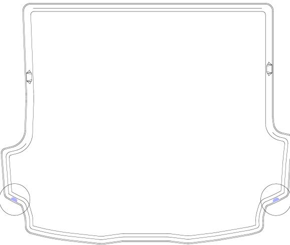
TO ACCESS THE FACTORY CARGO TIE DOWN HOOKS WITH YOUR LINER IN PLACE, TRIM AWAY THE MATERIAL FROM THE TWO LOWERED AREAS ON YOUR LINER (SHOWN ABOVE DARKENED) LEAVING THE RAISED EDGE. A UTILITY KNIFE WORKS WELL FOR TRIMMING.
