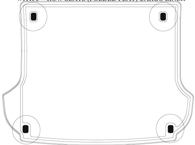
YOU CAN EASILY ACCESS THE FACTORY CARGO HOOK TIE-DOWN LOCATIONS IN YOUR SANTA FE WITH YOUR HUSKY LINER IN PLACE. TO DO SO, SIMPLY TRIM AWAY THE MATERIAL FROM THE 4 (FOUR) LOWERED AREAS IN YOUR CARGO LINER (SHOWN ABOVE CIRCLED AND DARKENED). A UTILITY KNIFE WORKS WELL FOR TRIMMING THESE AREA.USE CAUTION WHEN USING SHARP ITEMS SUCH AS A UTILITY KNIFE.
