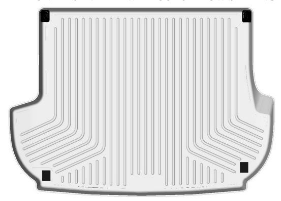
CARGO LINER PART #2792 IS DESIGNED TO ALLOW ACCESS TO THE FACTORY TIE-DOWN HOOK LOCATIONS WITH THE LINER IN PLACE. TO ACCESS THE HOOKS, YOU WILL NEED TO REMOVE THE MATERIAL FROM THE RECESSED AREAS OF THE LINER LOCATED DIRECTLY ABOVE THE HOOKS. THESE FOUR AREAS ARE RECESSED ON THE LINER TO AID TRIMMING. A UTILITY KNIFE WORKS WELL FOR TRIMMING.
