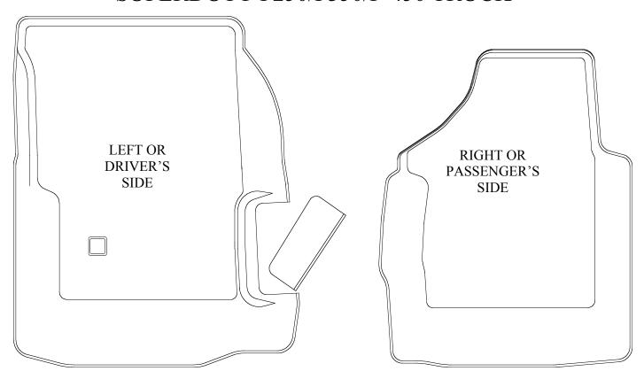
IF YOUR SUPER DUTY IS EQUIPPED WITH A MANUAL TRANSFER CASE SHIFTER, YOU WILL NEED TO TRIM YOUR LINER AS SHOWN ABOVE. TRIM AWAY THE MATERIAL FROM THE RAISED AREA ON YOUR LINER AS DEMONSTRATED ABOVE. A PHOTO OF THE TRIMMED LINER IS SHOWN ON THE BACK OF THIS PAGE. A UTILITY KNIFE OR HEAVY SHEARS WORK WELL FOR TRIMMING.
