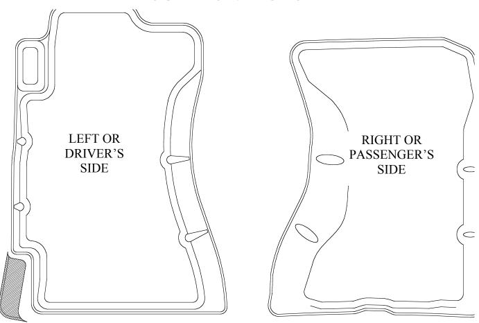
YOUR HUSKY LINER CAN EASILY BE TRIMMED TO ALLOW ACCESS TO THE FUEL DOOR RELEASE LEVER WITHOUT REMOVING YOUR LINER (FUEL RELEASE LEVER NOT USED ON ALL MODELS). TO ALLOW ACCESS, SIMPLY TRIM LINER USING THE MOLDED TRIM GROOVE AS A GUIDE. LEAVE THE \_" LIP AS DEMONSTRATED ABOVE.
