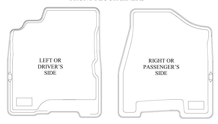
TO INSURE PROPER FIT OF YOUR DRIVER'S SIDE LINER, REMOVE THE TWO FACTORY CARPET HOOKS BEFORE INSTALLING YOUR LINER. THE CARPET HOOKS ARE EASILY REMOVED BY SIMPLY PULLING UP ON THE HOOK END. THE CARPET HOOKS WILL SNAP FREE FROM THE GROMMETS AND CAN BE STORED IN THE GLOVE BOX OR CONSOLE SHOULD YOU NEED TO REPLACE THEM AT A LATER DATE.
