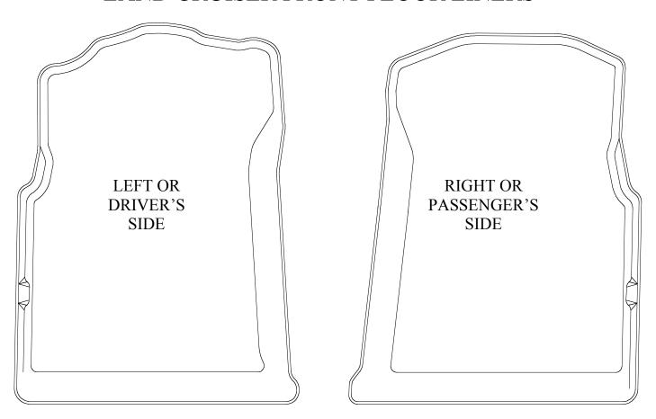
TO INSURE PROPER FIT OF YOUR DRIVER'S SIDE LINER, PLEASE REMOVE YOUR FACTORY CARPET HOOK. THIS CAN BE EASILY DONE BY PULLING THE L-SHAPED HOOK DIRECTLY TOWARD THE MOUNTING HOLE. THIS WILL ALLOW THE HOOK TO "POP" OUT. IT CAN BE STORED IN YOUR GLOVE BOX FOR REPLACEMENT AT A LATER DATE.
