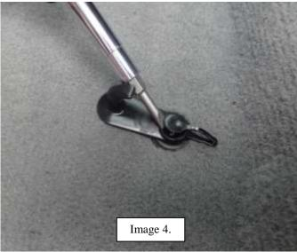
1) WITH THE FACTORY CLIPS REMOVED, UNSCREW THE TWO HALVES OF THE HUSKY® RETAINING CLIP AND INSERT THE BOTTOM HALF INTO THE EXISTING FACTORY GROMMETS LOCATION AS SHOWN BELOW IN IMAGE 4 AND IMAGE 5. THE BOTTOM PORTION WILL "SNAP" SECURELY INTO THE FACTORY GROMMET LOCATION. RETAIN THE TOP HALF OF THE CLIP FOR LATER INSTALLATION.
