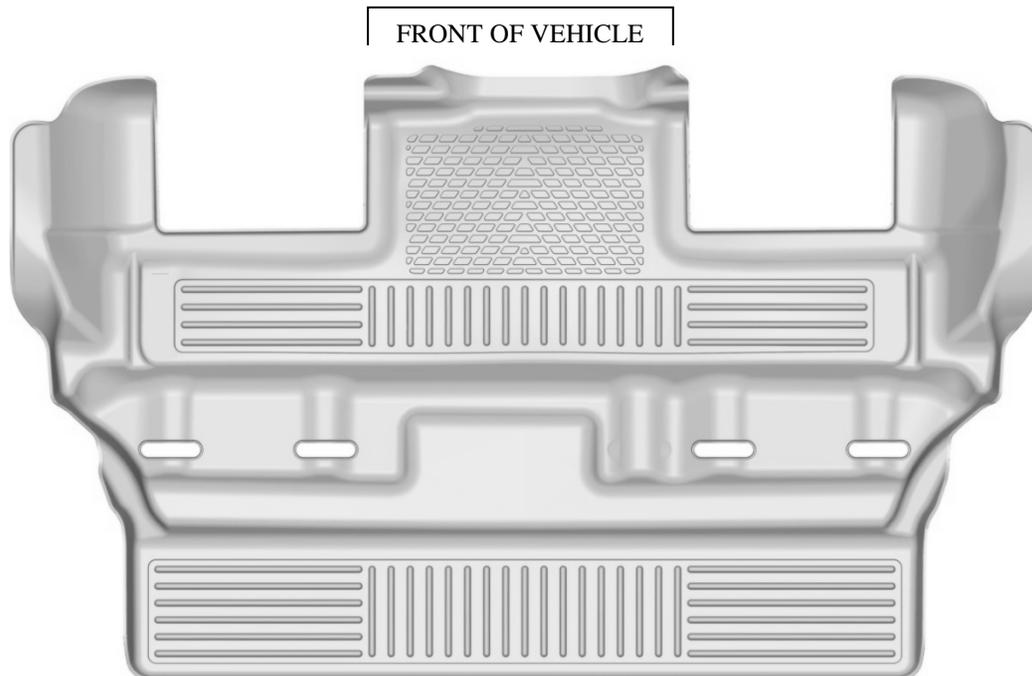
**BEFORE ATTEMPTING TO INSTALL YOUR LINER, FIRST FLIP/FOLD YOUR SECOND ROW BUCKET SEATS FORWARD TO EXPOSE THE 3<sup>RD</sup> ROW FLOOR PAN. WITH THIS DONE YOU CAN POSITION THE LINER IN THE FLOOR ORIENTED AS SHOWN ABOVE. THE “TONGUE” AREA PROVIDES COVERAGE BETWEEN THE 2<sup>ND</sup> ROW BUCKET SEATS AND TUCKS UNDER THE REAR EDGE OF YOUR 2<sup>ND</sup> SEAT LINER.**
