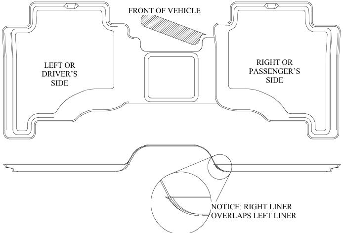
JEEP COMMANDER OWNERS WHOSE VEHICLE ARE EQUIPPED WITH THE FACTORY DVD PLAYER (ELECTRONIC INFOTAINMENT SYSTEM) WILL NEED TO TRIM THE CENTER HUMP PORTION OF THEIR DRIVER'S SIDE LINER TO ACCOMMODATE THIS OPTION. TRIM YOUR LINER AS SHOWN ABOVE USING THE MOLDED IN GROOVE AS A GUIDE (SEE PHOTOS ON BACK). A UTILITY KNIFE OR SCISSORS WORK WELL FOR TRIMMING.
