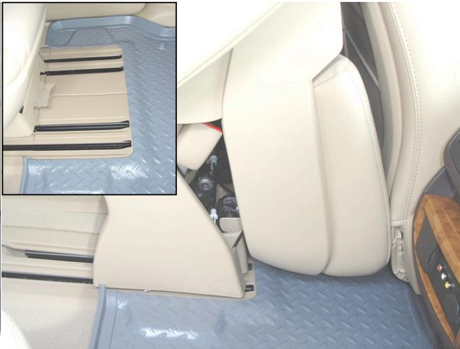
PART #6102 SHOWN TRIMMED TO ALLOW THE 2ND SEAT TO BE SLID FORWARD FOR MAXIMUM CARGO SPACE.
