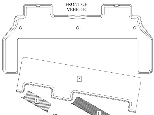
YOUR VEHICLE IS EQUIPPED WITH 2<sup>ND</sup> ROW BENCH ADJUSTED TO MULTIPLE POSITIONS. YOUR HUSKY TO ACCOMMODATE THESE POSITIONS VIA TRIM OPTIONS. SEATS POSITIONED FOR MAXIMUM 2<sup>ND</sup> ROW PASSENGER LEG FIT "AS BOXED". IF YOU WISH TO REPOSITION YOUR 2<sup>ND</sup> ROW SEAT PASSENGER LEG ROOM TRIM AWAY THE TREAD PLATED MAT
