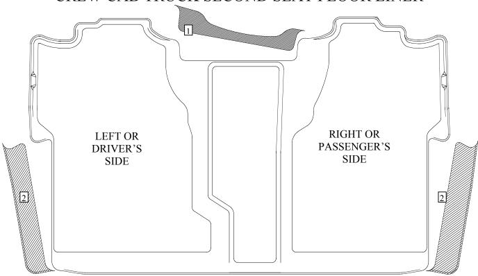
NOTE: IF YOUR TRUCK IS EQUIPPED WITH THE 40/20/40 FRONT BENCH SEAT, YOU WILL NEED TO TRIM AWAY A SECTION OF YOUR LINER. THIS IS EASILY DONE USING A UTILITY KNIFE OR PAIR OF HEAVY SHEARS. SIMPLY USE THE MOLDED IN GROOVE IN THE LINER AS YOUR TRIM GUIDE, REMOVING THE PORTION OF THE LINER ON THE "HUMP" PORTION OF THE LINER AS SHOWN ABOVE (SEE AREA "1"). MORE PHOTOS OF THE PART ARE ATTACHED ON THE BACK OF THIS PAGE.
