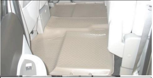
PART #6152 INSTALLED IN A CREW CAB TRUCK EQUIPPED WITH FRONT ROW CAPTAIN'S CHAIRS. NO TRIMMING IS NEEDED WITH THIS CONFIGURATION.
