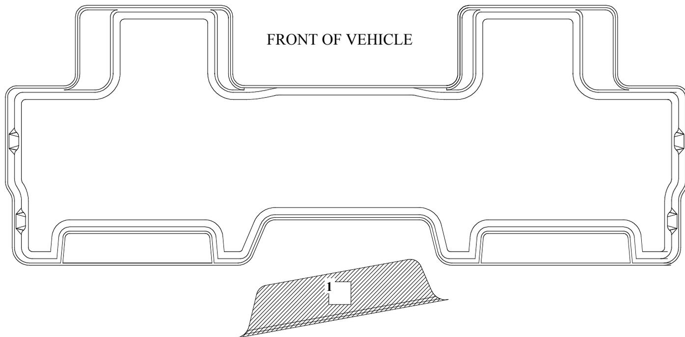
NAVIGATOR OWNERS WHOSE VEHICLES ARE EQUIPPED WITH THE SECOND SEAT CONSOLE WILL NEED TO TRIM THEIR LINER TO ALLOW FOR THE CORRECT FIT. TO TRIM, SIMPLY REMOVE THE TREADPLATED AREA FROM THE RAISED CENTER PORTION OF THE LINER (SEE AREA "1" ABOVE SHOWN CROSS HATCHED). USE THE EDGE OF THE TREAD AS YOUR TRIMMING GUIDE (SEE PHOTOS ON BACK). A UTILITY KNIFE OR HEAVY SHEARS WORK WELL FOR TRIMMING.
