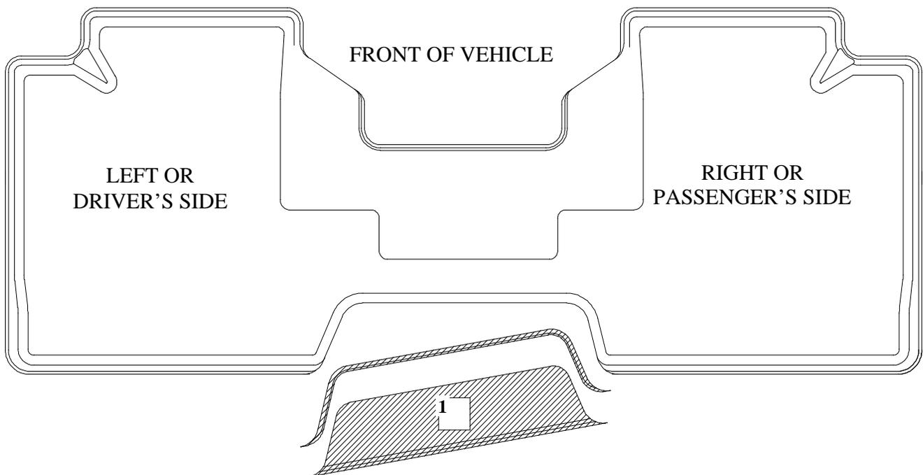
NAVIGATOR OWNERS WITH VEHICLES EQUIPPED WITH THE SECOND SEAT CONSOLE WILL NEED TO TRIM THEIR LINER TO ALLOW FOR THE CORRECT FIT. TRIM AWAY AREA "1" (SHOWN ABOVE CROSS HATCHED) BY USING THE MOLDED IN GROOVE. TRIM THROUGH THE REMAINING REAR WALL TO COMPLETE THE TRIM. A UTILITY KNIFE OR HEAVY SHEARS WORK WELL FOR TRIMMING.
