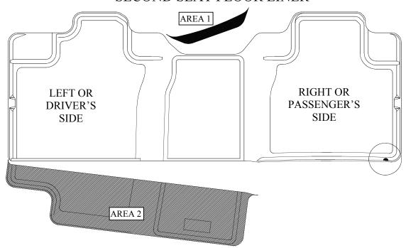
IF YOUR VEHICLE IS EQUIPPED WITH THE FACTORY 40/20/40 FRONT BENCH SEAT, IT WILL BE NECESSARY TO TRIM AWAY A PORTION OF THE LINER TO ACHIEVE THE PROPER FIT. TRIM BY REMOVING THE SMOOTH AREA (NO TREAD PLATE) OF THE LINER LOCATED ALONG THE FRONT EDGE OF THE PART AS SHOWN ABOVE (SEE AREA 1). A UTILITY KNIFE OR SCISSORS WORK WELL FOR TRIMMING. USE MOLDED IN GROOVE AS TRIMMING GUIDE (SEE PHOTOS ON BACK OF PAGE).
