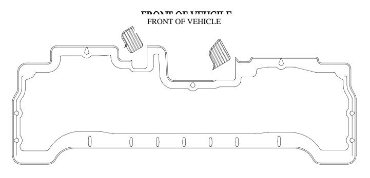
ON 1991 AND 1992 VEHCILES, SEAT BELT INTERFERENCE REQUIRES YOUR HUSKY LINER TO BE TRIMMED FOR PROPER FIT. TRIM AWAY THE AREA INDICATED IN THE ABOVE DIAGRAM. THIS AREA IS SLIGHTLY LOWERED ON THE LINER FOR EASIER IDENTIFICATION. TRIM WITH SCISSORS OR A UTILITY KNIFE.
