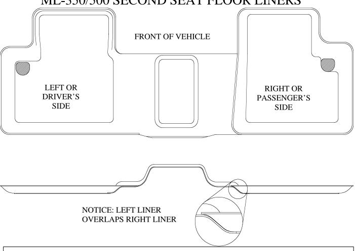
MERCEDES BENZ HAS LOCATED CARGO TIE DOWN HOOKS IN THE SECOND ROW FLOOR PANS. SHOULD YOU WISH TO ACCESS THESE CARGO TIE DOWN HOOKS WITH YOUR LINERS IN PLACE, SIMPLY TRIM AWAY THE MATERIAL FROM THE LOWERED AREAS ON YOUR LINERS SITUATED ABOVE THESE HOOKS (SHOWN ABOVE HATCHED). A UTILITY KNIFE WORKS WELL FOR TRIMMING.
