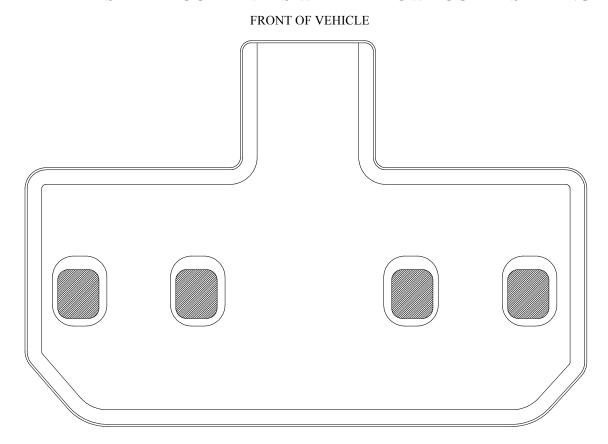
PLEASE FLIP/FOLD YOUR SECOND ROW SEATS FORWARD TO ALLOW INSTALLATION OF LINER. NOTE THAT THE FOUR AREAS SHOWN ABOVE DARKENED ARE TRIMMED TO ALLOW THE SECOND ROW SEATS TO FASTEN THROUGH THE LINER. IF YOUR LINER DOES NOT HAVE THESE FOUR AREAS TRIMMED, DO NOT INSTALL LINER AS YOUR  $2^{\rm ND}$  ROW SEATS WILL NOT FASTEN SECURELY. INSTEAD, PLEASE CALL HUSKY LINERS AT 800-344-8759.
