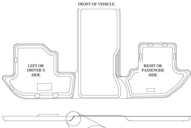
IF YOUR SUBURBAN OR YUKON XL IS EQUIPPED WITH THE 60/40 SPLIT SECOND SEAT, YOU MAY NEED TO TRIM YOUR LINER. REMOVE THE SHADED PORTION SHOWN ABOVE. A UTILITY KNIFE WORKS WELL FOR TRIMMING.
