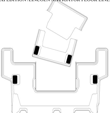
BEFORE INSTALLATION OF YOUR HUSKY LINER, CHECK LINER TO MAKE SURE THE FOUR (4) AREAS SHOWN ABOVE DARKENED ARE TRIMMED AWAY. IF THEY ARE NOT, DO NOT INSTALL LINER AS THE SECOND ROW OF SEATS WILL NOT LOCK SECURELY INTO POSITION. INSTEAD, PLEASE CALL HUSKY LINERS AT 800-344-8759.
