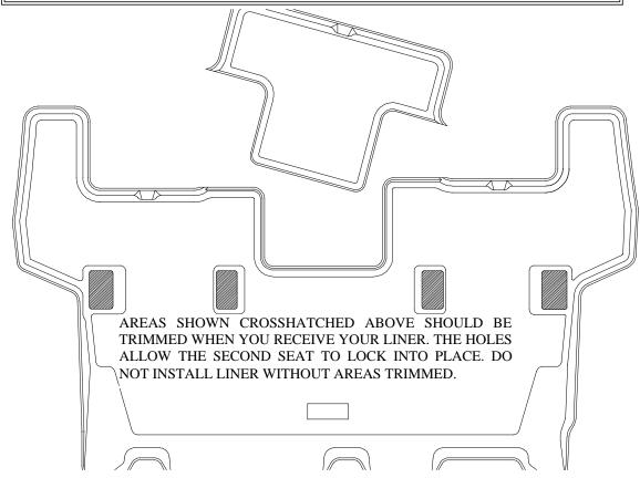
BEFORE INSTALLATION OF YOUR NEW HUSKY LINER YOU MUST FIRST RELEASE AND FLIP YOUR SECOND SEATS FORWARD. ALWAYS MAKE CERTAIN THAT THE SEATS ARE SECURELY LOCKED INTO POSITION BEFORE DRIVING VEHICLE.
