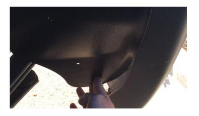
6. Insert the lower flap sections of the Wheel Well Guard into the fender well behind the fender well lip. Perform this step for both the front and rear lower flap sections. Well Guard lip is tucked behind the metal fender well lip of the truck
