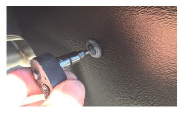
8. Install the factory Torx head screws at locations A, B, C, D, E and F.
