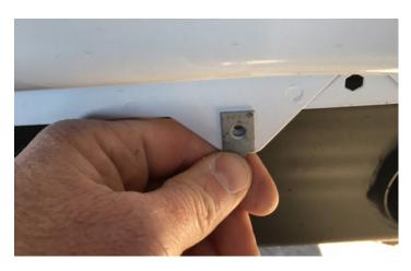
3. If your truck was not equipped with factory wheel well liners install a u-clip at locations C and D by clipping the u-clip over the tab and aligning with the factory hole.
