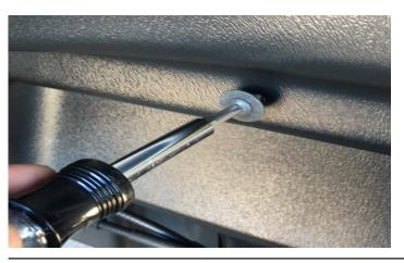
9. If your vehicle was not equipped with a factory wheel well guard, install the supplied SEM screws at locations C and D through the Wheel Well Guard and into the u-clips that are clipped over the sheet metal.
