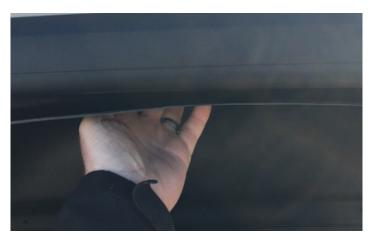
5. Push the Wheel Well Guard up into the fender opening.
