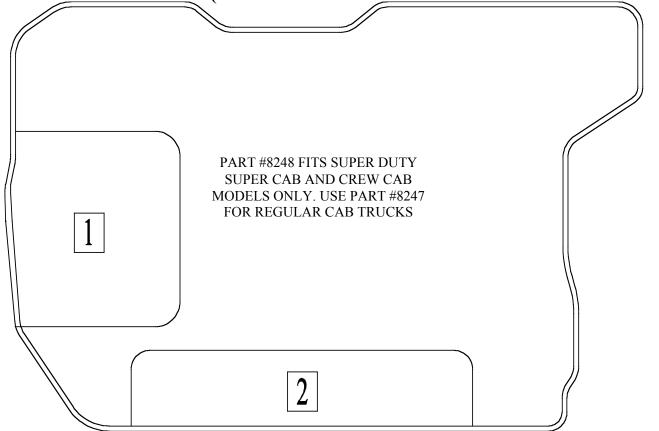
NOTE: IF YOUR VEHICLE IS EQUIPPED WITH A MANUAL TRANSFER CASE SHIFTER, YOU WILL NEED TO TRIM AWAY THE MATERIAL FROM AREA "1" SHOWN ABOVE. THIS AREA IS RECESSED ON YOUR LINER. USE THE EDGE FORMED BY THE RECESSED SECTION AS YOUR TRIMMING GUIDE. ONCE TRIMMED, THE LINER WILL FIT AROUND THE TRANSFER CASE SHIFTER HOUSING.
