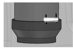
O Tack weld the Jounce Adapter (C) to the Chassis Tube (D) at each location. Make sure the adapter has remained fully seated against the tube before proceeding.
