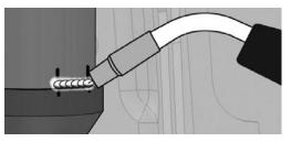
Allow the welded sections to cool and then drill a 3/8" hole through the Chassis Tube (D) immediately above one of the welds. HINT: The purpose of the hole is to facilitate the evacuation of any moisture that may collect inside the tube.
