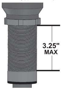
IMPORTANT: Internal threads of Jounce Adapter must remain fully engaged with Bump Shock Assembly at all times. Never operate vehicle when more than 3.25" of bump shock threads are exposed as illustrated above. Once the Bump Shock Assembly (A) is properly adjusted for your application, lock in place by turning the Bump Shock Nut (B) clockwise until it contacts the Jounce Adapter (C) and tighten. HINT: A spanner or strap wrench is useful for tightening Jounce Adapter Nut.
