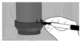
**HINT:** A pair of vertical lines spaced 0.5" apart is used to mark each weld location.
