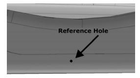
O Using the reference hole illustrated above as the center point, mark a 2.5" diameter circle on the bottom of the chassis rail. This indicates the material to remove in order to accommodate the supplied Chassis Tubes (D).
