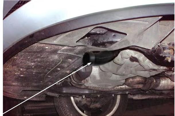
Taking all of the necessary safety precautions as per the manufacturers instructions, raise the front of the car. Pierce / drill two 3 mm holes in the under tray and plastic end of the cold air hose. Ovalise the end of the cold air hose and secure in position using the plastic ties supplied
