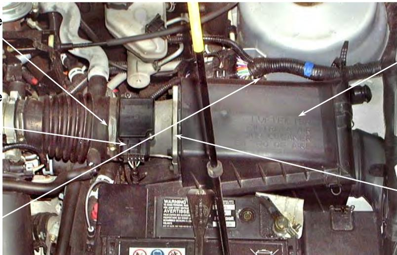
4. Lift the complete air box assembly out of its rubber mountings and remove it from the vehicle.
