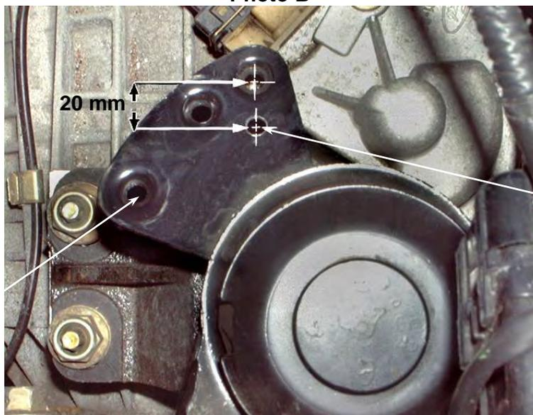
3. Drill an M6 clearance hole (6.5 – 7 mm) in the chassis mounted bracket as shown.
