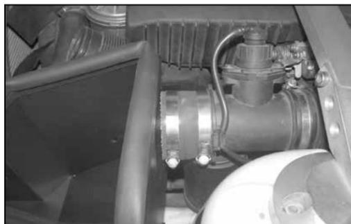
17. Install silicone hose (08690) onto the mass air sensor as shown with the provided hose clamps.
