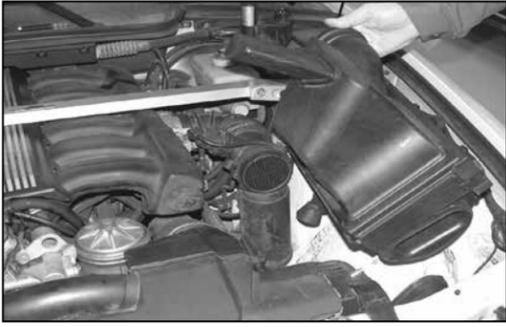
7. Remove the air box from the vehicle as shown.
