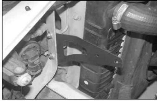
13. Install the heat shield mounting bracket onto the existing holes of the radiator core support with the hardware provided as shown.
