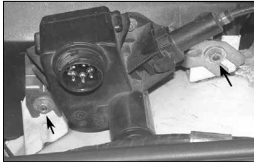
3. Remove the two speed control mounting nuts, then lift and place the speed control unit to the side.
