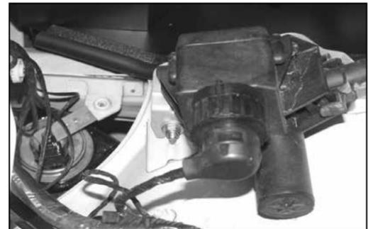
21. Reconnect the speed control electrical connection and twist the locking ring clockwise to lock in position.
