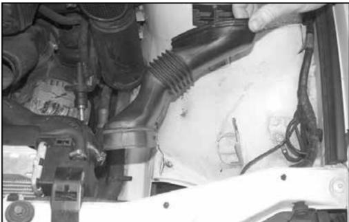
11. Remove the fresh air duct from the vehicle as shown.
