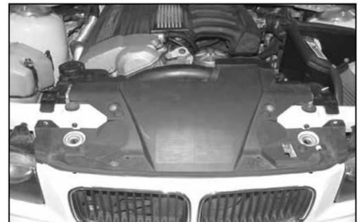
23. Re-install the radiator cover removed in step #9 and secure with the existing hardware.
