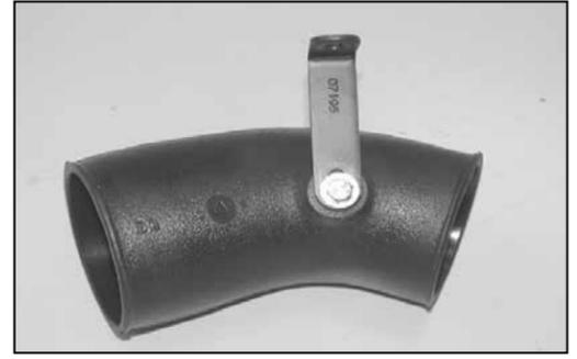
18. Install the tube mounting bracket (07195) onto the intake tube with the provided hardware.
