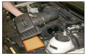
4. Loosen the hose clamp at the intake plenum and release the two clips that secure the air box lid to the vehicle. Remove the upper air box and intake tube as shown. 5. Remove the cover to the head light module to gain access to the air box bolts and module nut. Remove the bolts and nut.
