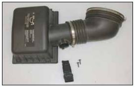
16. Remove the two screws that secure the mass air sensor to the air box with the provided Torx wrench, then remove the mass air sensor.
