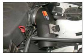
21. Attach the K&N $^{\!\!\rm ®}$  intake tube to the plenum with the provided hose clamp.
