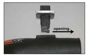
19. Install the mass air sensor assembly into the  $K\&N^{\ensuremath{\circledast}}$  intake tube.
