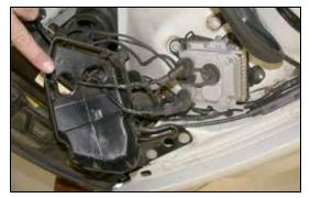
14. Re-install the head light module with the original hardware that was removed in step 5. **NOTE: Install provided spacer under front mount as shown, then re-install module cover.**
