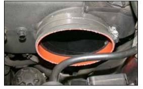
15. Install the silicone hose (08612) onto the intake plunem as shown using the provided hose clamps.
