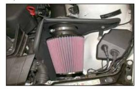
24. Install the K&N<sup>®</sup> air filter onto the K&N<sup>®</sup> intake tube and secure with the provided hose clamp.
