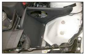
12. Install the heat shield into the vehicle. Make sure the lower air box mounting studs protrude through the heat shield mounting holes.
