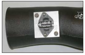
20. Secure the mass air sensor assembly into the K&N $^{\circ}$  intake tube with the provided hardware as shown.
