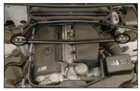
2. Remove the four 13mm nuts that secure the strut tower brace to the vehicle, then remove the brace from the vehicle.
