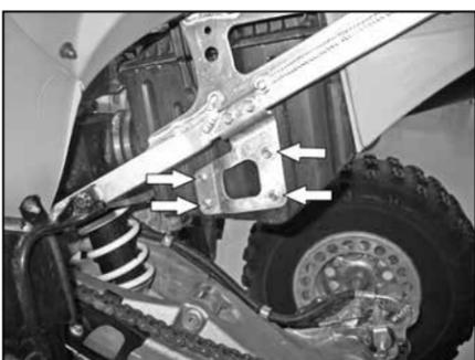
4. Remove the eight bolts which secure the factory air box to the frame side mounts, there are four bolts on the left side and four bolts on the right side of the air box.
