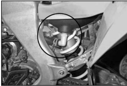
18. Install the 90° vent fitting into the K&N® intake tube as shown. Then connect the factory crank case vent hose to the fitting and secure with the factory clamp.
