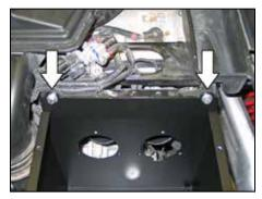
16. Secure the top of the air box to the mounting bracket with the provided hardware and then tighten the lower mounting nut and hose clamp securing the fresh air intake hose.
