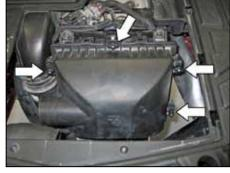
4. Loosen the five air box retaining nuts and release the retaining nuts.
