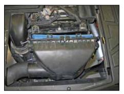
5. Depress the two locking tabs and then remove the air box half from the vehicle.
