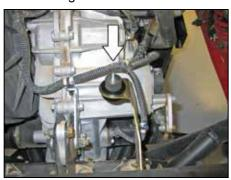
12. Install the rubber mounted stud onto the heat shield mount as shown.
