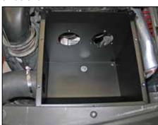
15. Install the air box into the vehicle so that the stud protrudes through the hole on the bottom and the fresh air supply hose is installed onto the air box tube. Then install the lower mounting hardware but do not completely tighten at this time.
