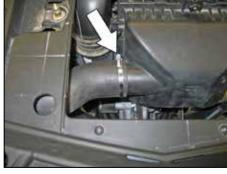
3. Loosen the hose clamp securing the fresh air intake hose to the air box and then disconnect the fresh air intake hose from the air box.
