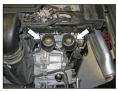
13. Install the silicone hoses (08476) onto the throttle bodies and secure with the provided hose clamps.
