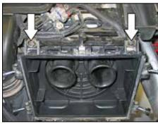
7. Remove the two bolts securing the air box to the mounting bracket.
