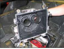
9. Remove the air box half from the vehicle as shown.
