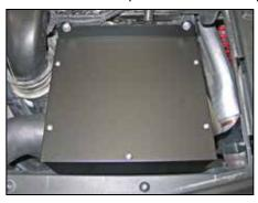
22. Install he air box lid and secure with the provided hardware.
