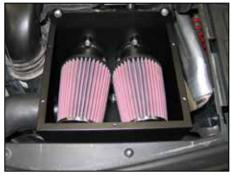
21. Install the K&N® air filters onto the intake tubes and secure with the provided hose clamps.
