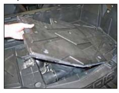
2. Remove the engine access panel from the cargo bay.
