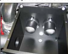
20. Install the left side intake tube (27548) through the heat shield and into the silicone hose on the throttle body, and then secure with the provided hardware and hose clamp.
