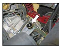
11. Assemble the heat shield mount onto the air box mounting bracket.
