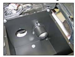
17. Install the right side intake tube (27547) through the heat shield, rotate 180\* and then install into the silicone hose at the throttle body. Secure the intake tube with the hose clamp and hardware provided.
