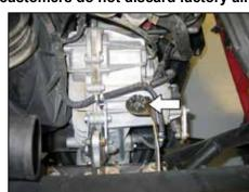
10. Remove the lower air box mounting grommet shown.
