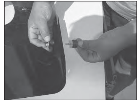
8. Install the two rubber isolator stand off using the provided hardware as shown.
