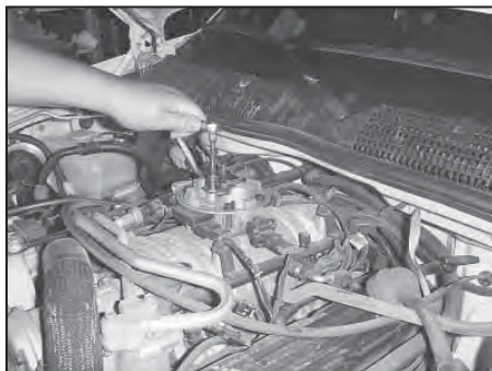
7. Using a 7/16" socket, loosen and remove the stud assembly as shown.
