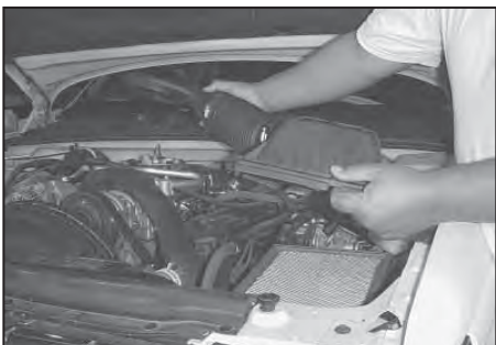
4. Unclip the six over center clamps and remove complete upper intake assembly as shown.
