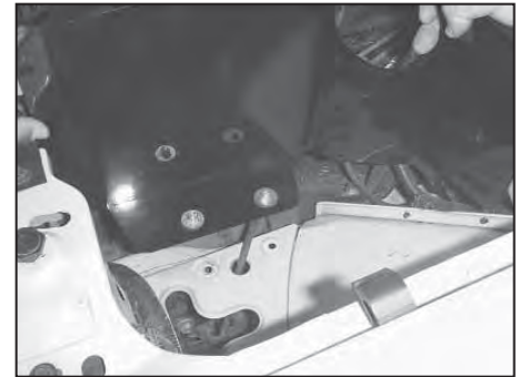
10. Install the heat shield with the hardware provided.
