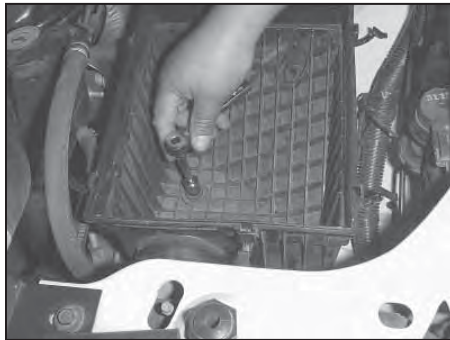
5. Using a 1/2" socket, loosen and remove the three bolts that secure the airbox base.
