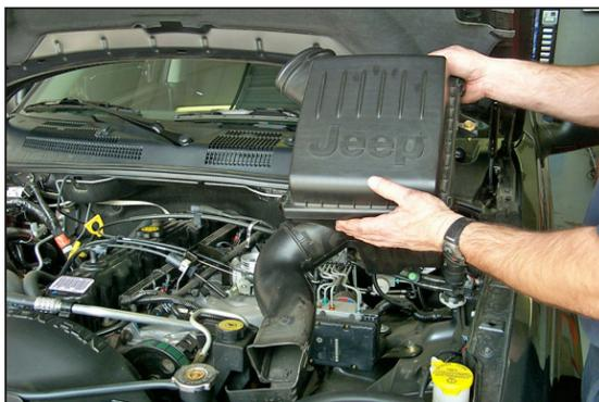
5. Remove the three nuts that secure the air cleaner assembly from underneath the vehicle, then, remove the air cleaner assembly as shown. **NOTE: K&N Engineering, Inc., recommends that customers do not discard factory air intake.**
