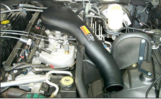
11. Install the K&N® intake tube into the silicone hose as shown, but do not tighten completely as some adjustment may be necessary.
