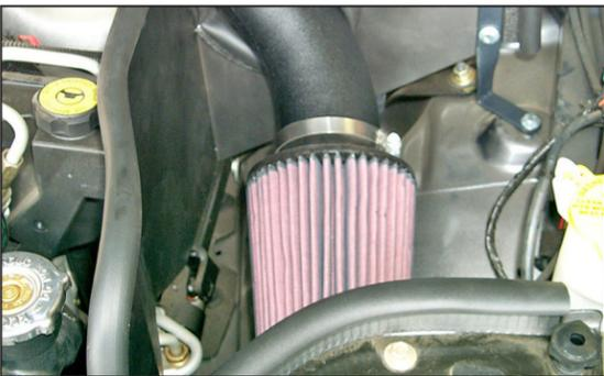
13. Install the K&N® Air Filter onto the K&N® intake tube and secure with the provided hose clamp.
