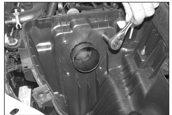
7. Remove the four throttle body to air box retaining bolts as shown.
