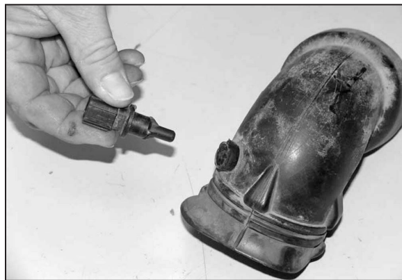
4b. Remove the clamp, which secures the air temperature sensor to the fresh air intake, and then remove the air temperature sensor as shown.
