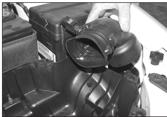
4a. Pull up to remove fresh air intake from the inner fender.
