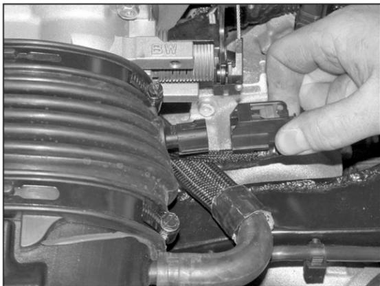
2. Disconnect air temp sensor electrical connection.
