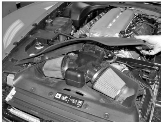
4. Loosen the six airbox cover screws and remove airbox lid.
