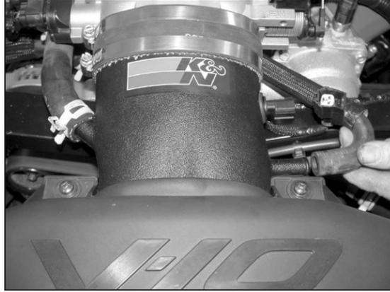
14. Install idle air hose and crank case vent hose onto K&N intake tube as shown.
