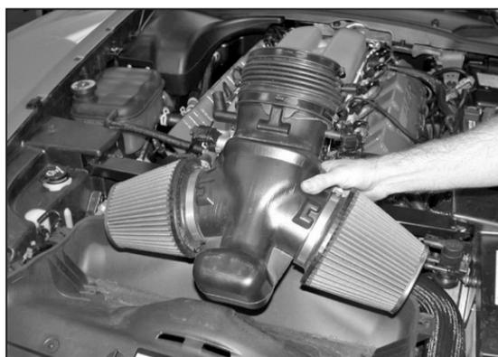
5. Loosen intake tube hose clamp at throttle body, and remove wing nut under tube. Then remove complete intake assembly.
