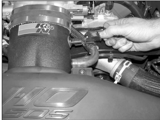
15. Reconnect air temp sensor electrical connection.
