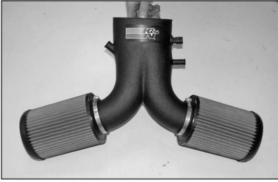
10. Install the air filter onto the K&N® intake tube.
