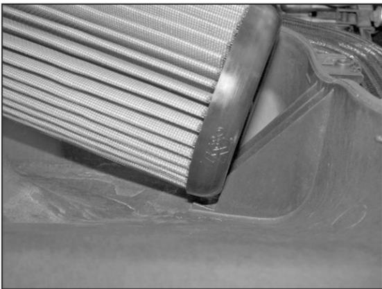
11. Install the K&N® intake assembly onto the vehicle as shown.
