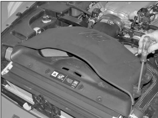
12. Reinstall upper airbox cover removed in step #4 and tighten six mounting screws.
