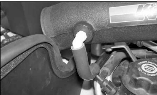
26. Install cut crankcase vent hose onto the NPT fitting as shown.
