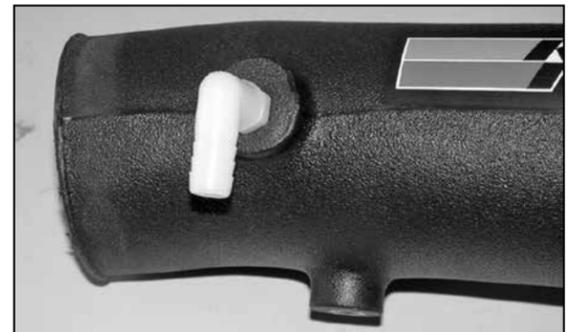
22. Install the 90° NPT fitting into the K&N® intake tube as shown.
