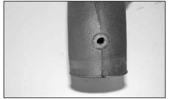
19. Install the provided grommet in the K&N® intake tube as shown.
