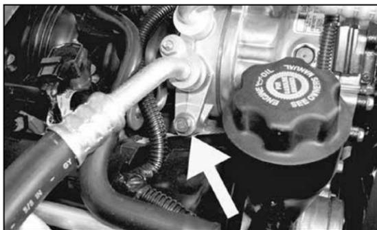
17. Remove the A/C compressor-mounting bolt.
