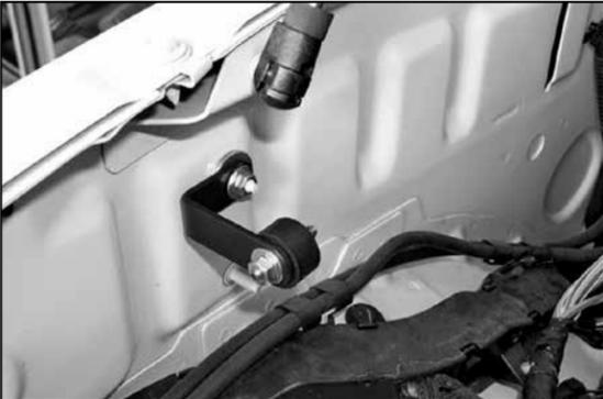
9. On vehicles that do not come with TCM's mount "L" bracket onto existing stud with the provided hardware.
